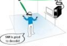
Figure 5—MoVR's setup: The PC is connected to a mmWave AP and the headset is equipped with a mmWave receiver. In the case of a MoVR user, user turns her head, the AP steers its beam towards the MoVR reflector. The reflector amplifies the signal and reflects it toward the headset.
